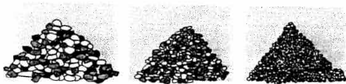
Figure 3-4: Aggregates of different sizes are blended with fines.
